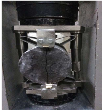
Figure 6 Split tensile strength test setup
