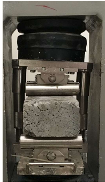
Figure 9 Flexural strength test setup
