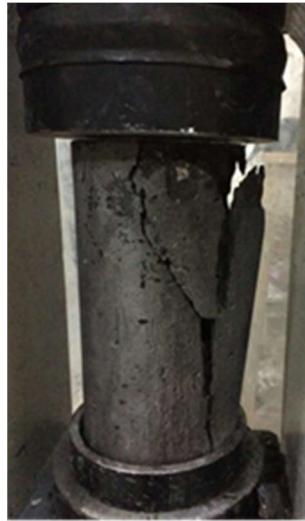
Figure 3 Compressive strength setup
